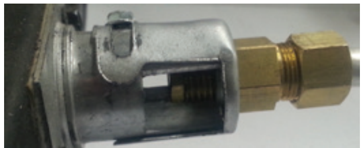
Figure 3 - Air Shutter Fully Open
